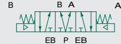
double air pilot 3 Position 4-Way (5/3), open to 4 (A) and 2 (B) in center
